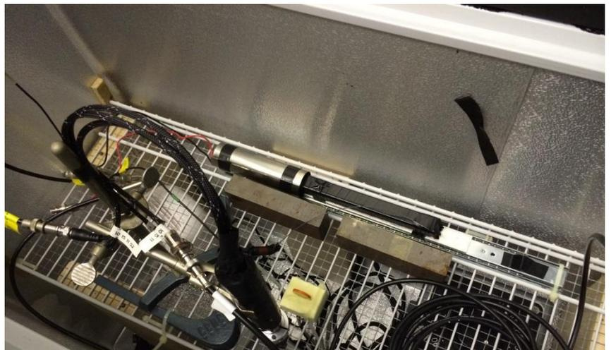
Figure 5: Set up for measuring light yield. The radioactive source is on the yellow styrofoam. The two iron bricks are the collimator. The crystal and PMT are in center back wall. The trigger PMT and scintillator are center front wall. Beneath the setup is the heater and a dehumidifier which stops ice from forming on the walls.
