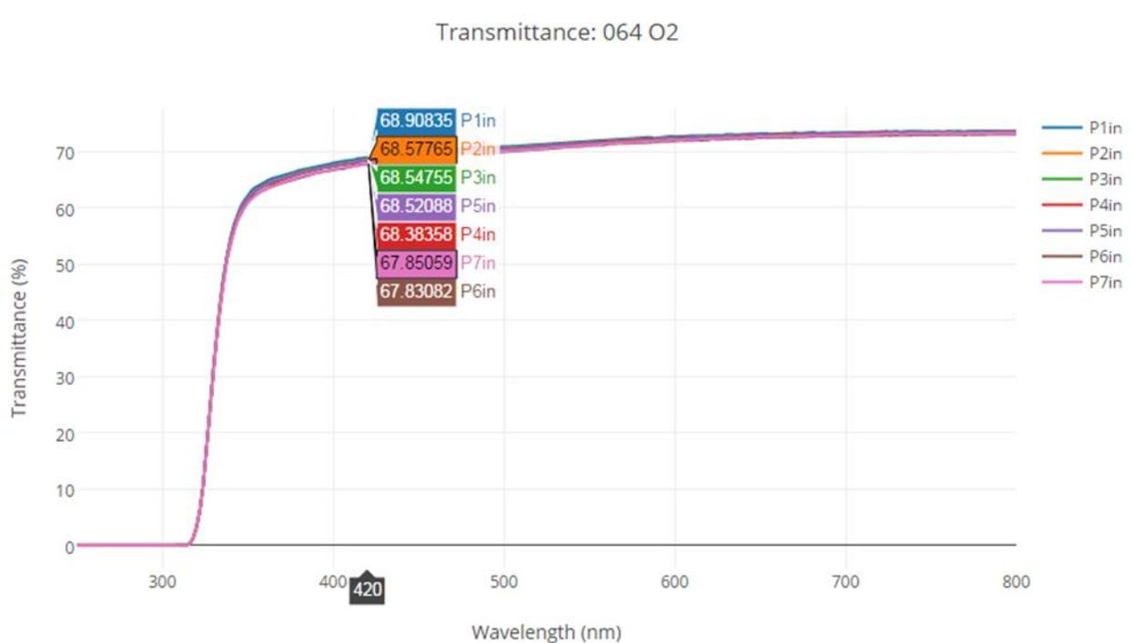
Figure 16: There is clearly a deviation between the two orientations here. Also, interestingly, there again is a trend of higher transmittance from one end of the crystal to the other.
