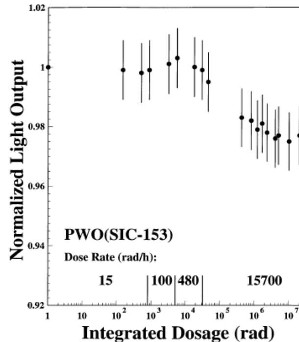
The light response uniformity as a function of the integrated dose for PbWO<sub>4</sub> (From R.-Y. Zhu, NIM, A413, p297, 1998)
