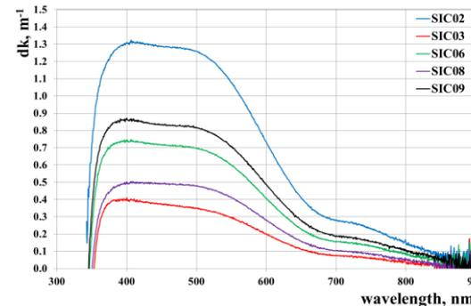
Irradiation tests performed in collaboration with Giessen university show SIC produced crystals are radiation hard
