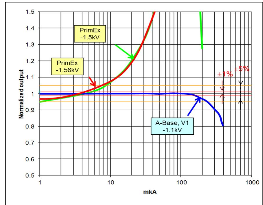
Active base equivalent output integral current is about 400 mA and outperforms PrimEX passive base by factor of ~25
